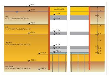
Figure 1. Cross section of the two-level underground car park - steel sheet pile solution (design by Witteveen & Bos).
