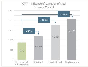
Figure 7. Global Warming Potential – Total (t of  ${\rm CO_2}$ -eq.) – Scenario with corrosion of steel sheet piles.
