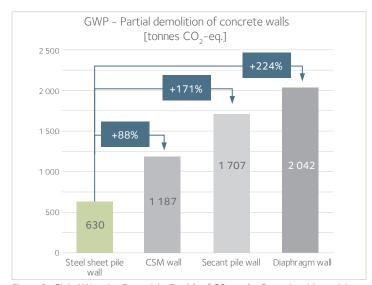
Figure 8. Global Warming Potential - Total (t of CO<sub>2</sub>-eq.) - Scenario with partial demolition of the diaphragm wall and secant pile wall.
