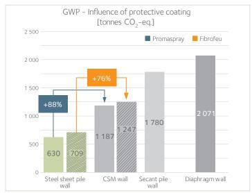
Figure 10. Global Warming Potential – Total (t of CO<sub>2</sub>-eq.) – Influence of the fire protection system (paintings).
