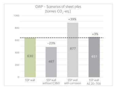
Figure 11. Global Warming Potential - Total (t of CO<sub>2</sub>-eq.) – Influence of the scenarios on the GWP of the steel sheet pile wall.
