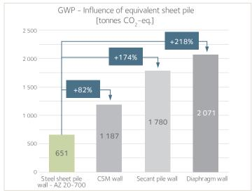
Figure 9. Global Warming Potential – Total (t of  $CO_2$ -eq.) – Scenario with the equivalent sheet pile profile AZ 20–700.
