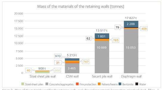
Figure 2. Mass of the materials used for the retaining walls, excluding soil movements (excavation, mixed soil, back-filling,...).
