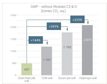
Figure 6. Global Warming Potential - Total (t of CO<sub>2</sub>-eq.)-Scenario without modules C3 and D.
