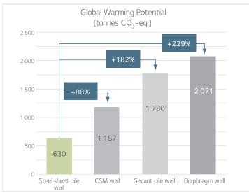
Figure 3. Global Warming Potential - Total impact for the UCP (t of CO<sub>2</sub>-eq.).
