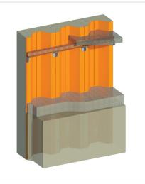
b. Horizontal slab on a steel support
