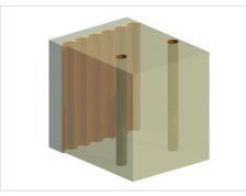
a. Steel sheet piles & piles for foundations installed
