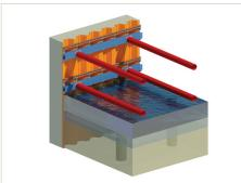
d. Installation of bottom strut, excavation under water, followed by bottom slab poured under water
