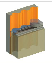
b. Impervious connection with bottom slab, solution 2
