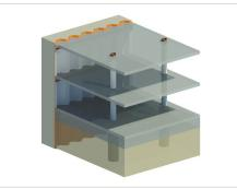
f. Execution of permanent slab (acting as strut) and removal of top strut
