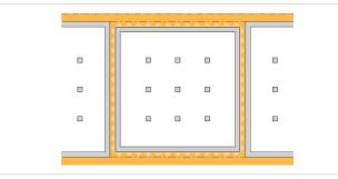
b. Steel sheet piles for temporary use, pulled-out after execution of concrete structure
