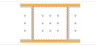
a. Steel sheet piles for temporary and permanent use (gain in surface)
