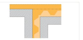
Arcelor Mittal developed several sealing systems to reduce the seepage through the interlocks.
