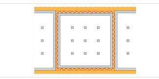
c. Steel sheet piles for temporary use, stay in place after execution of concrete structure
