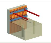
c. Installation of top strut, followed by excavation to level slightly below second strut
