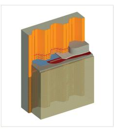
a. Impervious connection with bottom slab, solution 1
