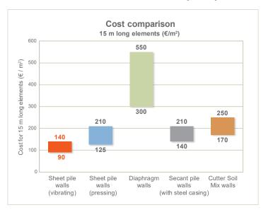
A steel sheet pile wall is up to 50% more cost-effective than a secant pile wall.
