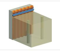
b. Excavation to level slightly below top strut
