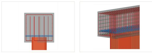
Fig. 2. Capping beam with typical reinforcing bars (based on the German National Technical Approval)
