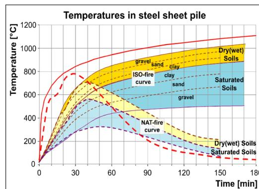
Fig. 2: Temperatures in steel sheet piles based on different fire design curves.
