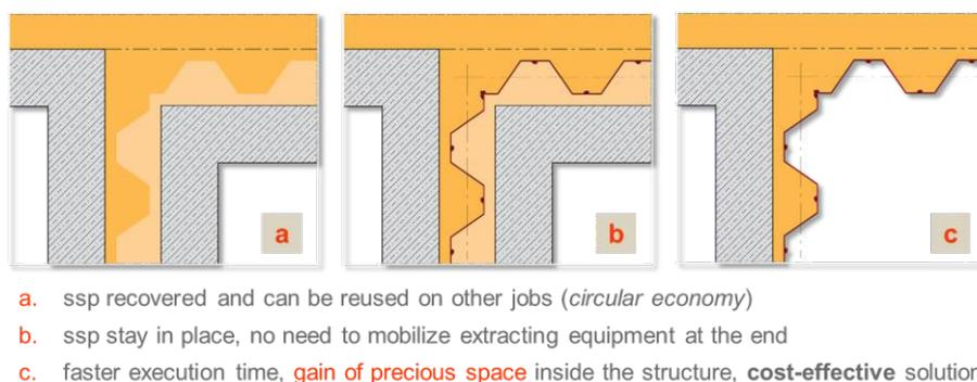
*Fig. 2: Execution options for a UCP. Plan view.*
