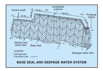
The base seal is connected to the vertical enclosure wall by means of serrated plates welded to the steel sheet piling; a PEHD strip is
