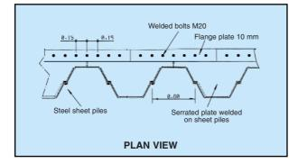
fixed to the serrated plates by means of a loose flange. The strip is connected to the general PEHD seal.
