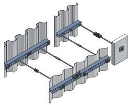
Steel Z-pile with spherical nut (articulated)
