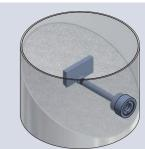
Combi & D-wall cast-in spherical box A machined 'spherical box is cast into the tube transferring forces to the centre of the tube. Forged spherical anchor bars are connected to the box allowing articulation in both the vertical & horizontal directions.
