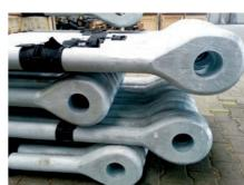
With the exception of ASD0700 bar Anker Schroeder tie bars and components can be hot dip galvanised to EN ISO 1461 but consideration should Anker Schroder can offer factory petro- be given to threads which are unable to have more than a nominal coating of zinc. Please contact our technical department for further detail.
