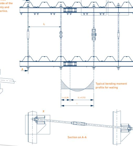
Anchor connections to a sheet pile wall can be made in two ways – outside the wall or inside as shown opposite. Generally walings placed inside the retaining wall are preferred both for aesthetic reasons and, in the case of a wall in tidal or fluctuating water level conditions, to prevent damage to the waling by floating craft or vice versa.
