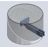
Combi wall cast-in T-Plate A fabricated T-Plate is cast into the tube transferring forces to the centre of the tube. Forged eye anchor bars are attached to the T-connector via a pin allowing articulation in the vertical direction. See table 7 for more detail.
