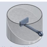
Combi wall - cast-in forged eye A forged eye bar is cast into the tube transferring forces to the centre of the tube. The anchor bars are attached to the cast-in bar via link plates allowing articulation in the vertical direction.
