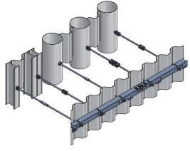
Anchor forces are generally high and articulated connections
