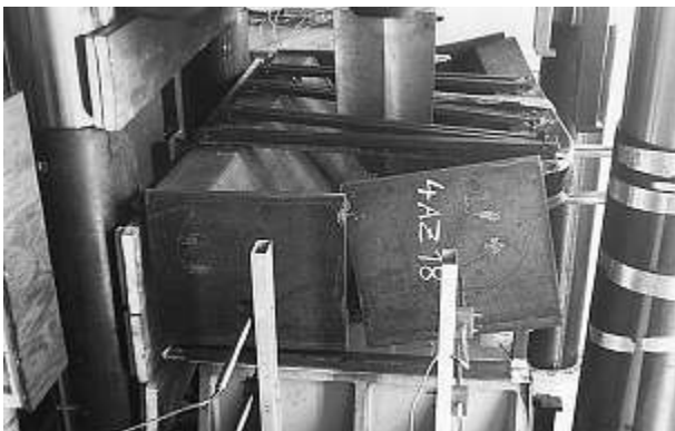
Double AZ18 sheet pile during test
