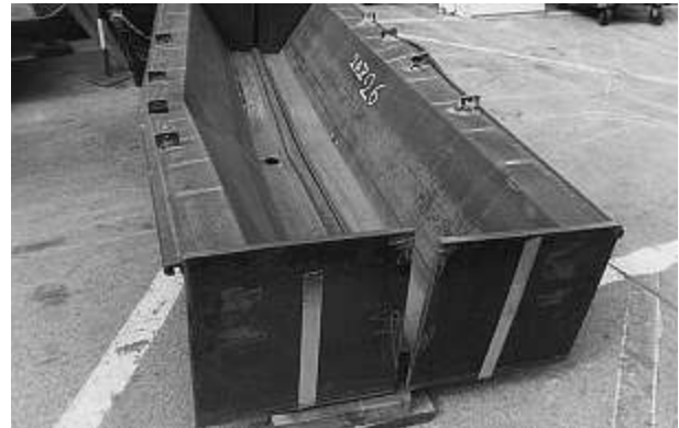
Double AZ18 sheet pile after test
