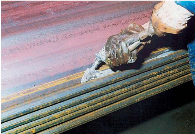
Workshop installation of the waterswelling sealing system
