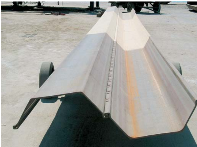
A three-layer coating system was applied on the waterside of the steel wall
