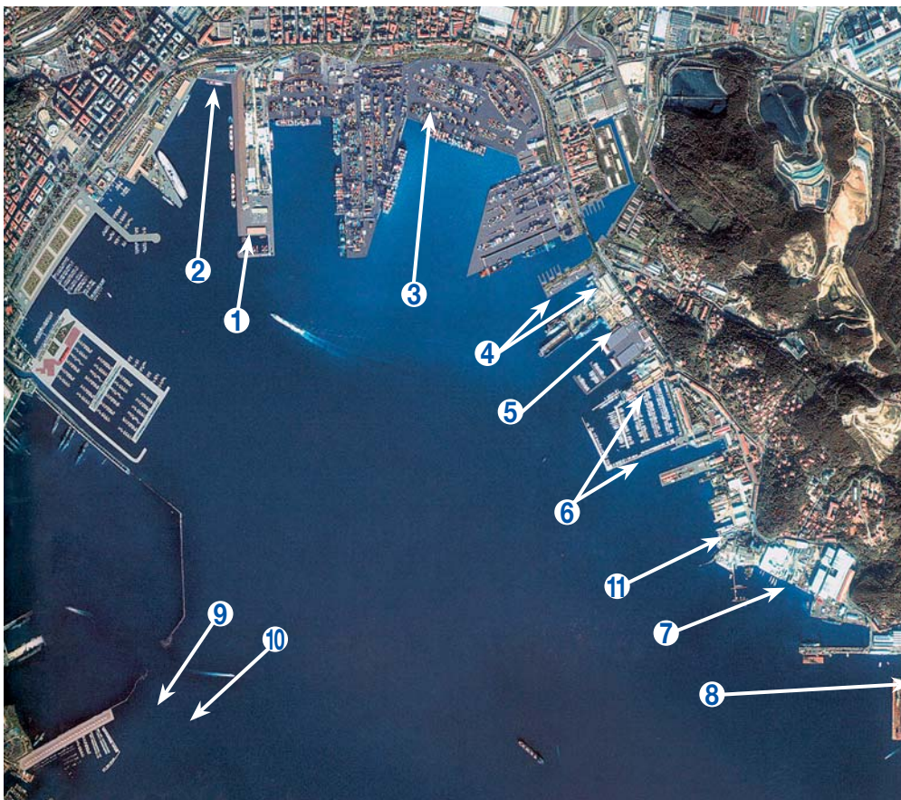
27,500 t of sheet piles were used for eleven projects in La Spezia
