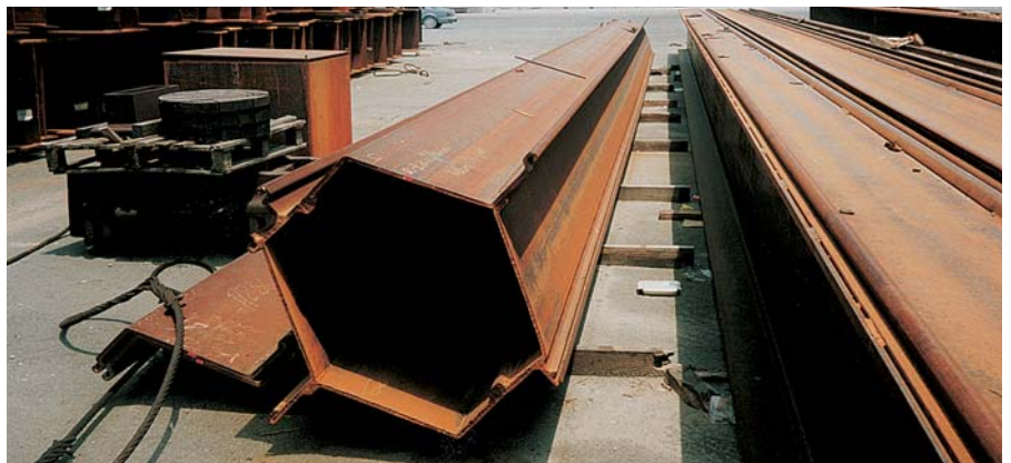
A CAZ 36 box pile with three interlocks welded on was used where the anchor walls intersect
